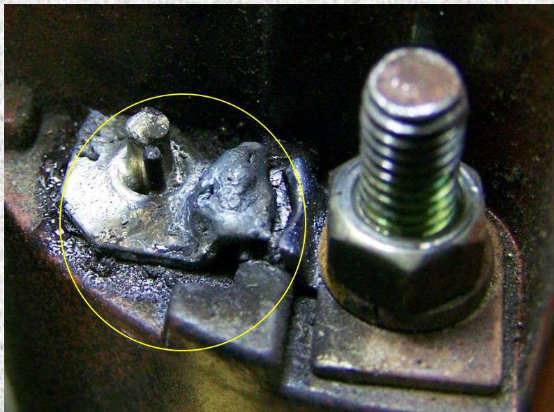
Solder re-flow due to excessive heat
