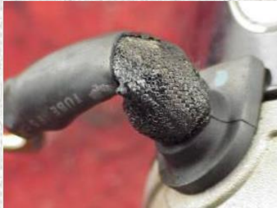
Motor strap insulator discolored by over-crank.
