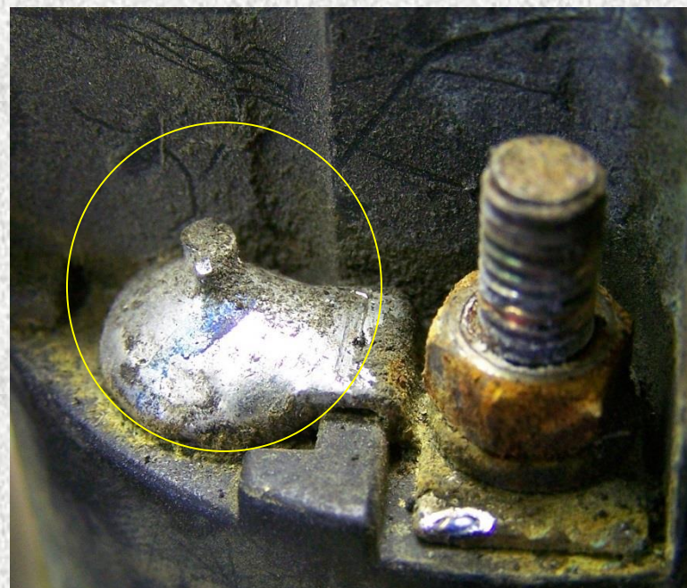
Good Solder on Solenoid
