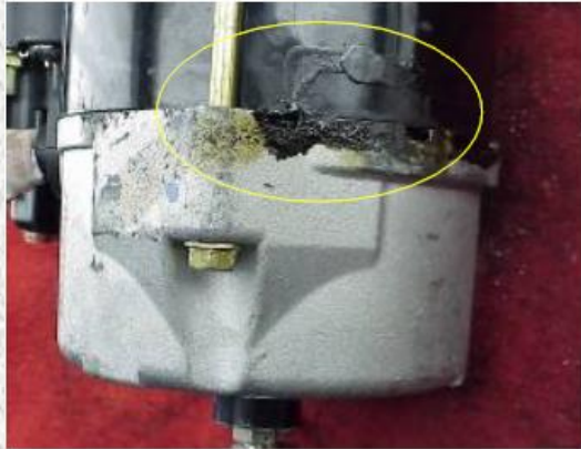
Melted varnish will flow from the starter and become black from heat.
