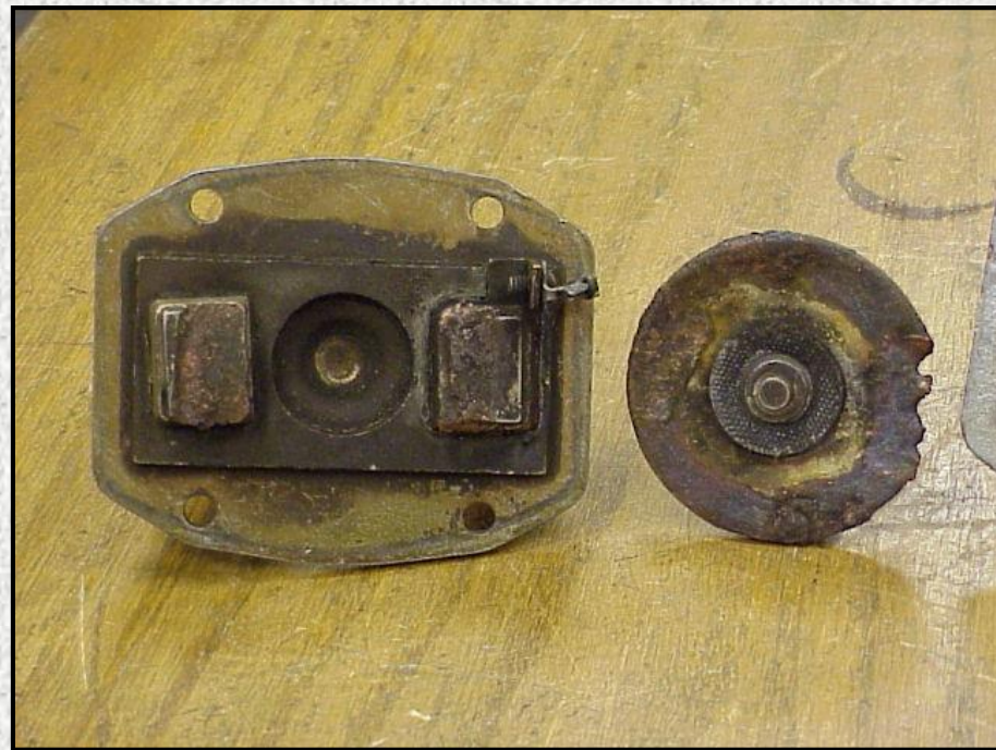
Damaged – Caused by low system voltage
