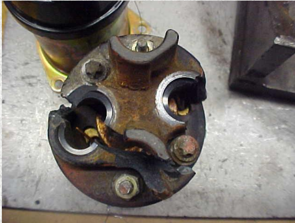
Solenoid Cap : Fractured
