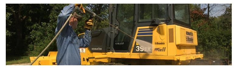
While both the Delco Remy branded starters and alternators are laboratory tested to withstand salt spray, muddy water, dust, high pressure water and chemical exposure, it's important to avoid contamination during cleaning. Direct exposure of the starter or alternator to high pressure water, steam or chemical cleaners will shorten the service life of these electrical products by increasing circuit resistance and heat.
