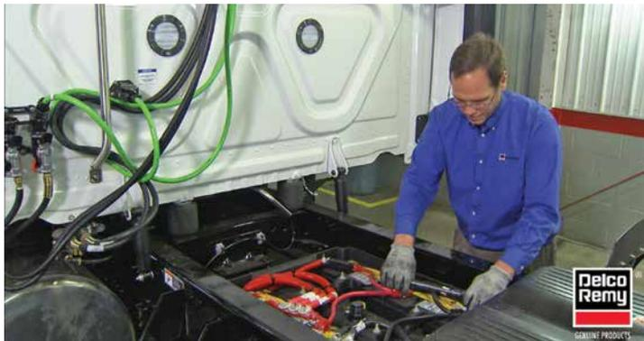
Complaints can arise when heavy current demand conditions exist. Sometimes there are resistance losses in the power cables which, in turn, limit the regulated voltage available—sometimes by as much as a half-volt. This results in lower battery state-of-charge and less efficient operation.
