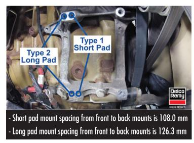
The corresponding holes on the pad mount alternator may be larger in diameter. This allows variations in the bracket and alternator assembly. These holes are mainly for securing the alternator in position.
