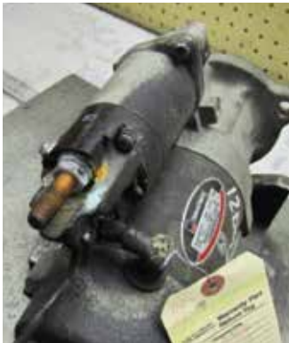
Missing IMS switch
