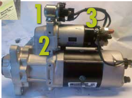
The switch will be located on one of three mounting locations just forward of the solenoid. Notice the wires that come off of the switch.
