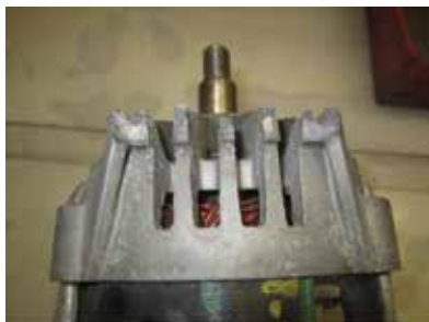
Mounting ear completely broken off
