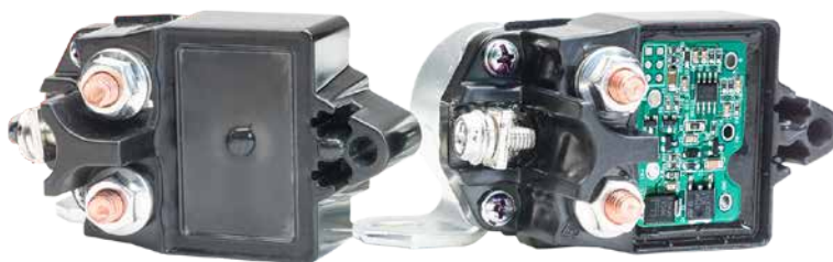
Programmable Printed Circuit Board (PCB) connected to the IMS
