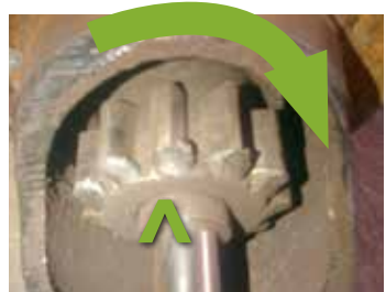
All teeth show damage from being run into a running engine.
