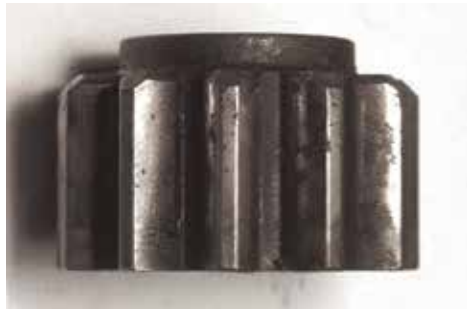
Normal wear marks showing over \frac{3}{4} of the drive surface being used.
