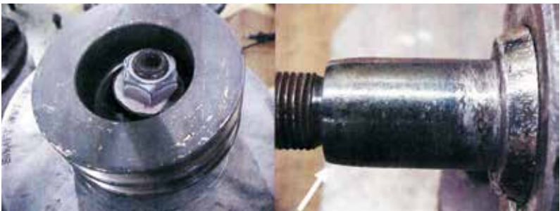
Examples of loose pulley damage on external fan type alternators
