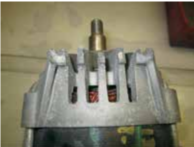
Mounting ear completely broken off
