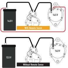
Remote Sense utilizes a second wire that reads the actual voltage at the battery. This signals the alternator to boost its output to compensate for the voltage drop, ensuring 14 Volts at the battery. The proper voltage forces more current into the battery bringing it to a full state of charge between vehicle stops.
