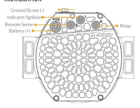
NOTE: When the Remote Sense terminal is not connected, the alternater operates and regulates voltage normally.
